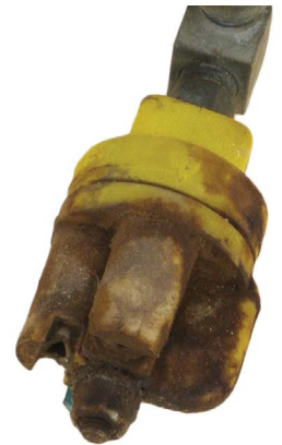
This nozzle is clogged!!!!
